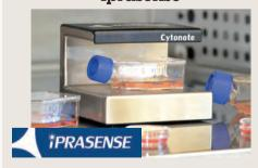
Lensless imagery technology that enhances tenfold the visual field compared with a microscope and video capture solutions for monitoring growth of cell cultures without marking.
